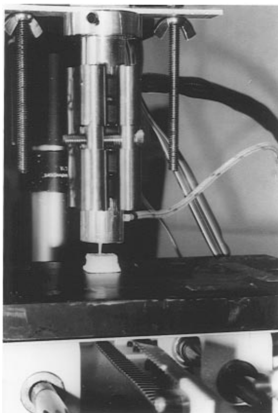
Figure 2. Reactive extrusion free-forming equipment. (a, top) Moving head writing ceramic slurry onto a stationary substrate. (b, bottom) Fixed, heated, head writing onto a motorized table.
